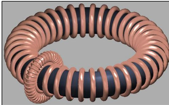
Figure 10. Additive coil added on.
