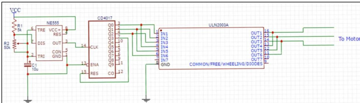
Figure 1. DC circuit design (lines going to the motor are going to the individual coil packs, possibly in pairs)
