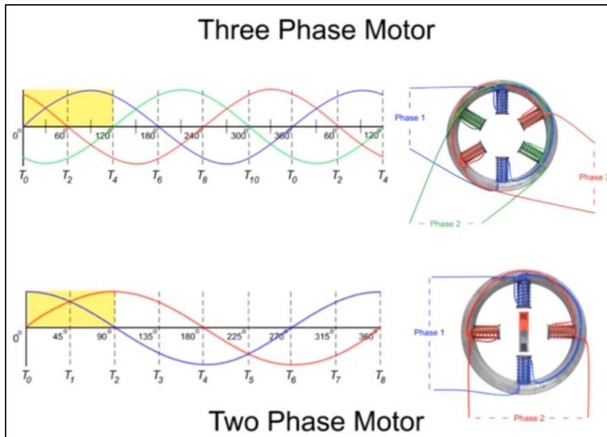
Figure 3. Difference between 2 and 3 phase AC motors. Both are feasible.
