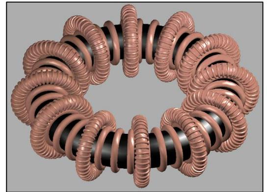
Figure 7. Torus surrounded by many additive coils.
