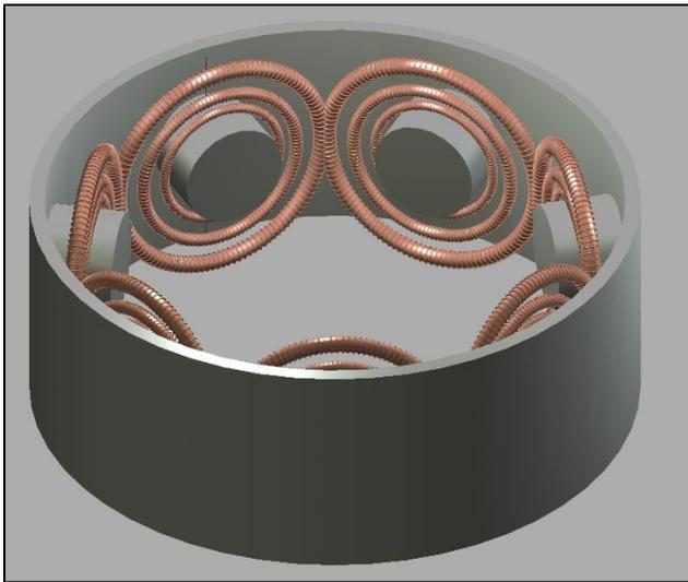
*Figure 4. Cylinder structure with coils on the inside.*
