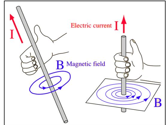
Figure 15. Shows how the right-hand rule can be used to determine current and magnetic field directions.
