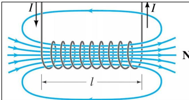
Figure 14. Magnetic field lines shown in blue, with a current running through the wire shown in grey.
