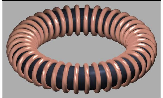
Figure 8. Torus surrounded by insulated copper wire.
