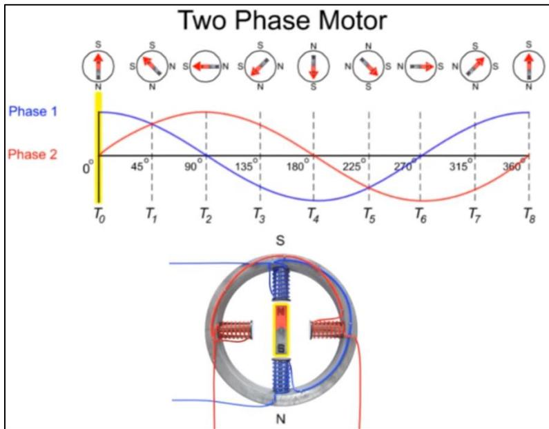
Figure 2. Possible 2 phase motor utilizing AC
