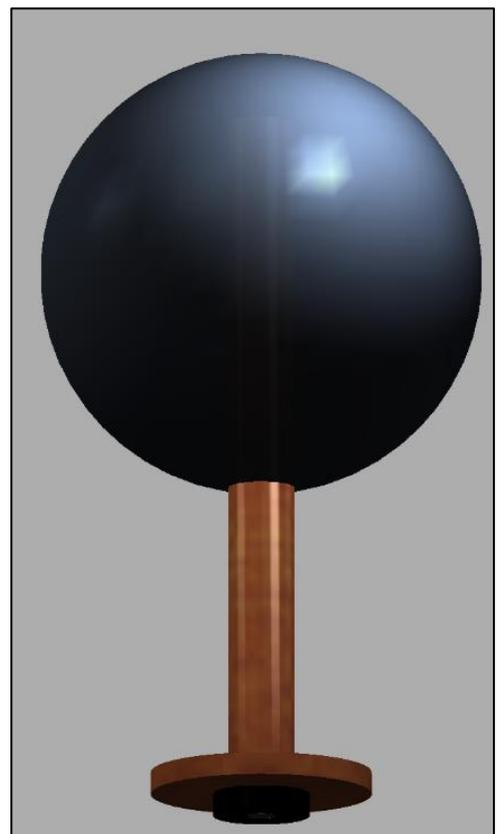
*Figure 5. Sphere of ferrofluid supported on a stand with a bearing underneath for possible rotation.*
