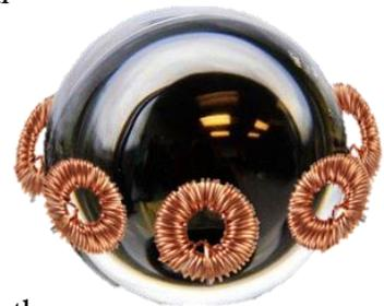
*Figure 1. Ferrofluid container surrounded by inductors.*
